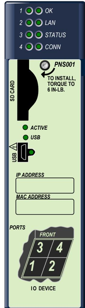
**Note:** Under certain ambient operating temperatures, the PROFINET Scanner could momentarily display the over temperature pattern during power up, while it is calibrating its thermal protection functions. This indication can be ignored. For details, see “Microprocessor Over Temperature” in the *PACSystems RX3i PROFINET Scanner Manual*, GFK-2737.
