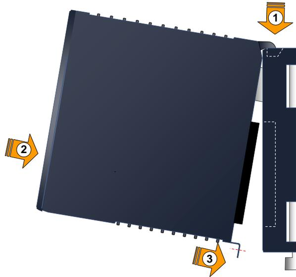
**3. Connecting the PNS to the PROFINET network and to a 10BaseT, 100BaseTX or 1000BaseT IEEE 802.3 network for general Ethernet communications**
