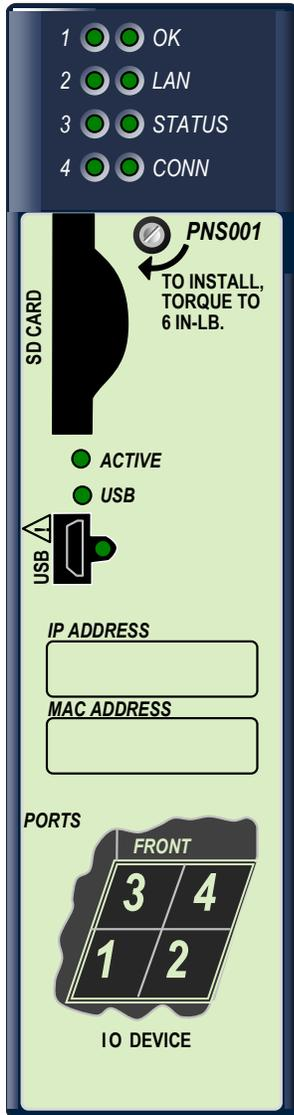
The PACSystems\* RX3i PROFINET Scanner (PNS) module, IC695PNS001, connects a remote universal RX3i I/O rack of Series 90-30 or RX3i modules to a PROFINET IO-Controller. The PROFINET Scanner scans the modules in its rack, retrieving input data and providing output data, and exchanges that data on the PROFINET IO LAN at the configured production rate.
