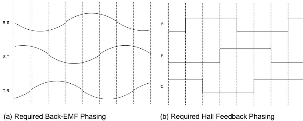
Many motor manufacturers include drawings in their data sheets that identify the phasing of the back-EMF and Hall feedback signals, or an application engineer may have access to an internal document listing the information. As a last resort, the motor can be rotated in the lab to check the phasing.
