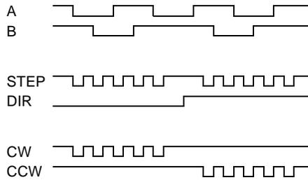
The ULTRA 200 Series drive may be electronically geared by a remote signal. Electronic gearing may be driven by any of the following three signals:
