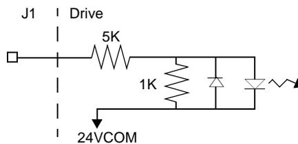
Two discrete input circuit types are available on the J1 connector. Both circuits support logic type interfaces with 24 Volt, optically isolated, single ended and active high, current sinking characteristics.
