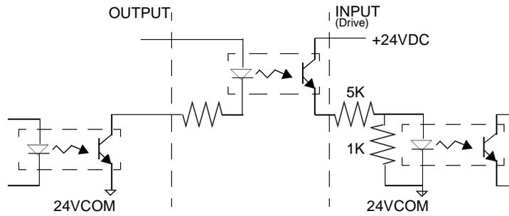
**Figure 6.7 Drive Input Connected to Sourcing Output**
