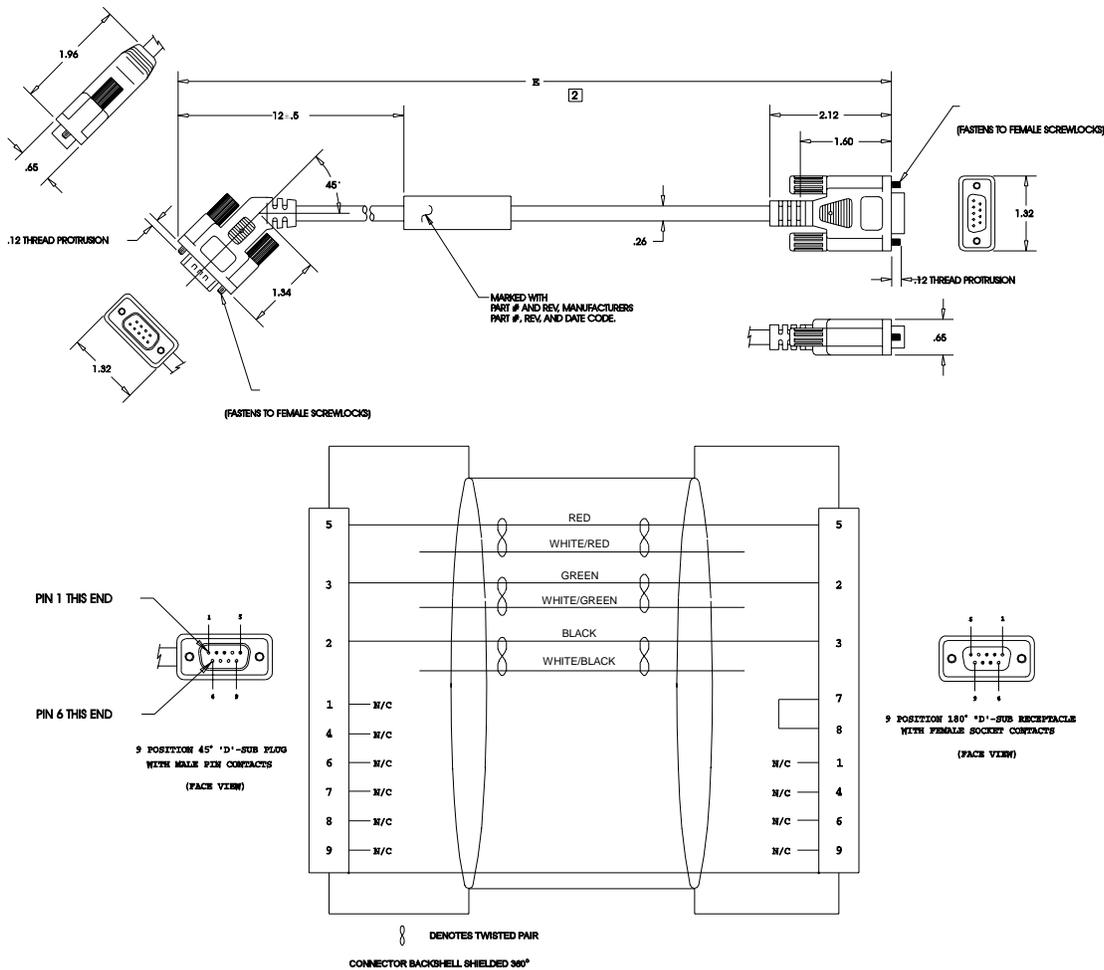
Figure B.10 J5 to J5 Serial Interface Cable (P/N 9101-1374)
