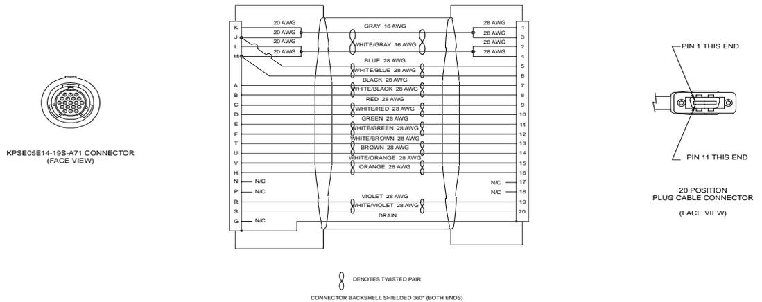
Figure B.18 No Connector to N-Series Encoder Cable (P/N 9101-1469)
