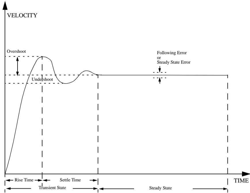
Figure 9.4 Underdamped Signal
