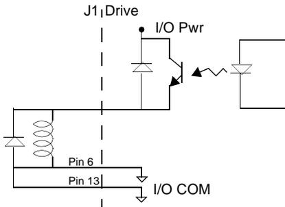
**Figure 6.14 Drive Output Connected to Active Low Input using a Switch/Relay**
