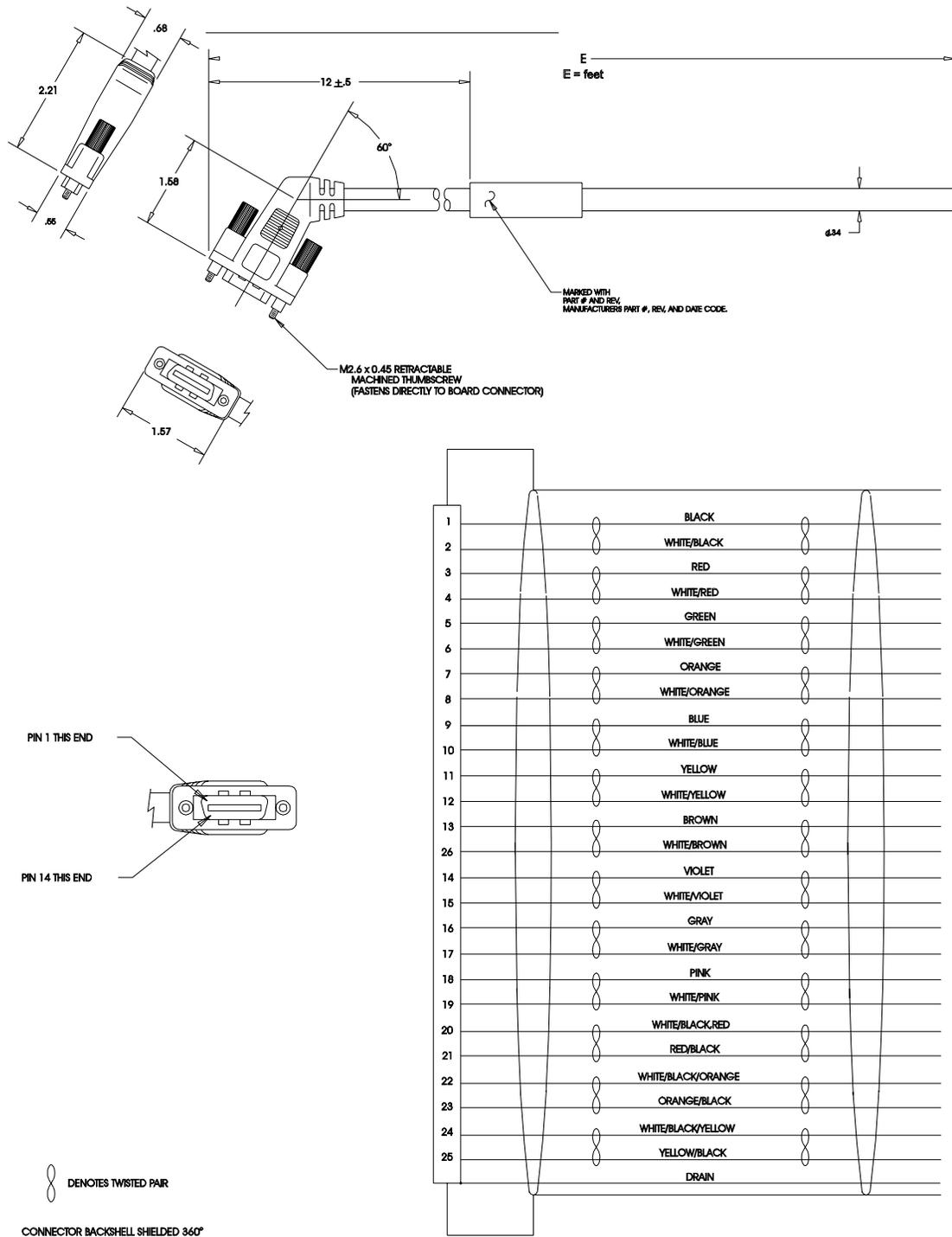
**Figure B.5 J1 to 50-pin Terminal Block Kit Diagram
