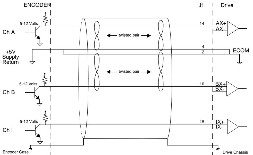
Figure 6.29 Single-Ended Encoder Interface via Open Collector Transistor with 24 VDC Pull-up (not recommended)
