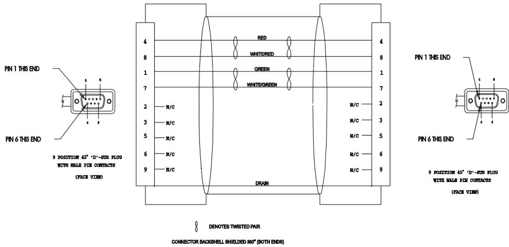
Figure B.11 J5 to No Connector Serial Interface Cable (P/N 9101-1379)
