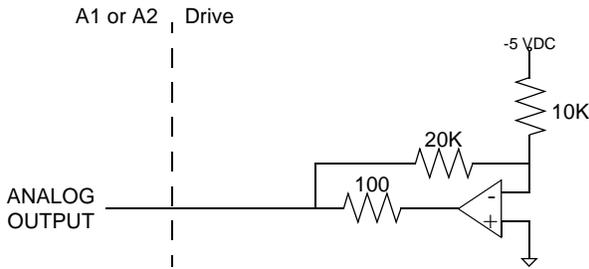
A 12-bit digital-to-analog converter (DAC) generates ANALOG 1. ANALOG 2 is a filtered PWM signal with 8 bit resolution and a carrier frequency of 32.8 kHz. Both outputs are scaled to a range of -10 to +10 Volts.
