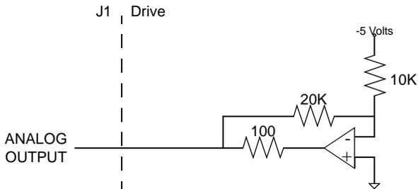
Two selectable outputs are available for monitoring by the user: ANALOG 1 (J1-30) and ANALOG 2 (J1-31). A 12 bit digital to analog converter (DAC) generates ANALOG 1. ANALOG 2 is a filtered PWM signal with 8 bit resolution and a carrier frequency of 32.8 kHz. Both outputs are scaled to a range of -10 to +10 Volts.
