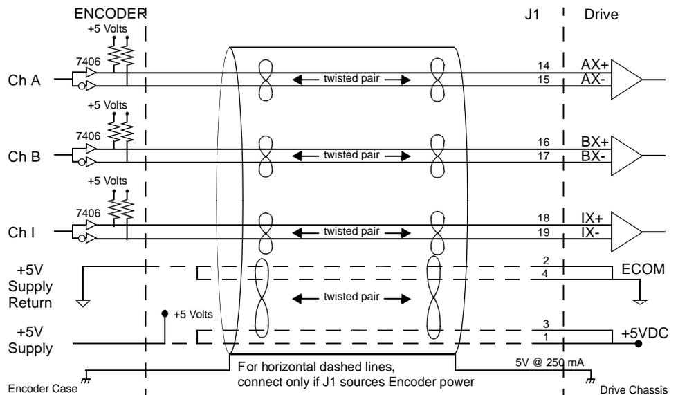
Figure 6.25 Complementary Encoder Interface via Standard TTL Logic
