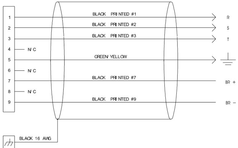
Figure B.25 N-Series Power Cable (P/N 9101-1467)
