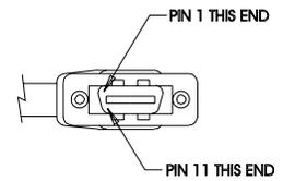
Figure B.15 No Connector to Y-Series Encoder Cable (P/N 9101-1373)
