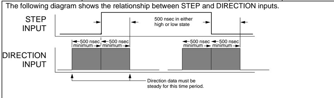
Figure 6.30 External Step/Direction Interface via TTL Differential Line Drivers
