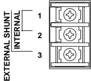
The shunt regulator is enabled when the DC bus increases to a specific value (420 VDC). An increase in DC bus voltage always occurs when the drive decelerates the motor and its load. This is due to the current flow from the motor to the DC bus. When the energy transferred from the rotating inertia causes the DC bus voltage to exceed 420 VDC the shunt is enabled and the excess energy (>420 VDC) is dissipated as heat.
