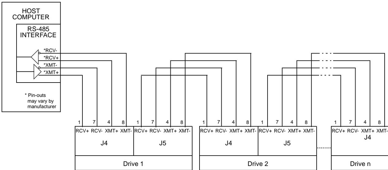
Multiple axes systems may be controlled by a computer with an RS-232 serial port. An RS-232 serial communication port may be converted to four wire RS-485 communication by attaching an RS-232 to four wire RS-485 converter. The figure below depicts the use of such a device. A daisy chain wiring configuration may also be used as shown in Figure 6.41.
