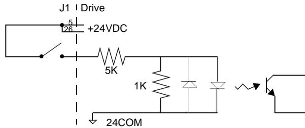
Figure 6.3 Drive Input Connected to an Opto-Isolator
