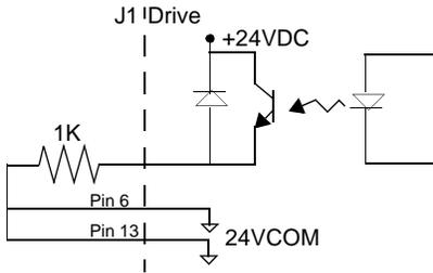
Figure 6.13 Drive Output Connected to a Switch/Relay
