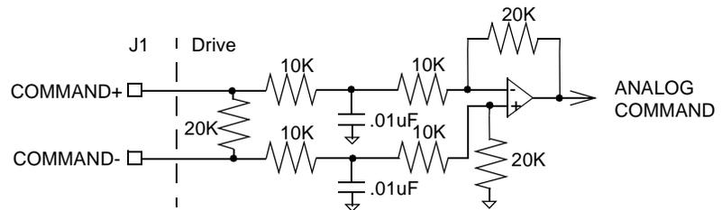
The analog command signal to the drive has a range of  $\pm 10$  Volts. The signal is either a torque, velocity or position command, depending on the software configuration of the drive. The differential input is processed by a 16 bit analog to digital converter (ADC) to produce a digital value.
