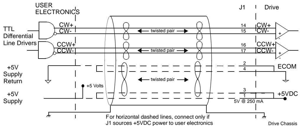
Figure 6.33 External CW/CCW (Step Up/Step Down) Interface via Single-Ended Line Drivers (not recommended)
