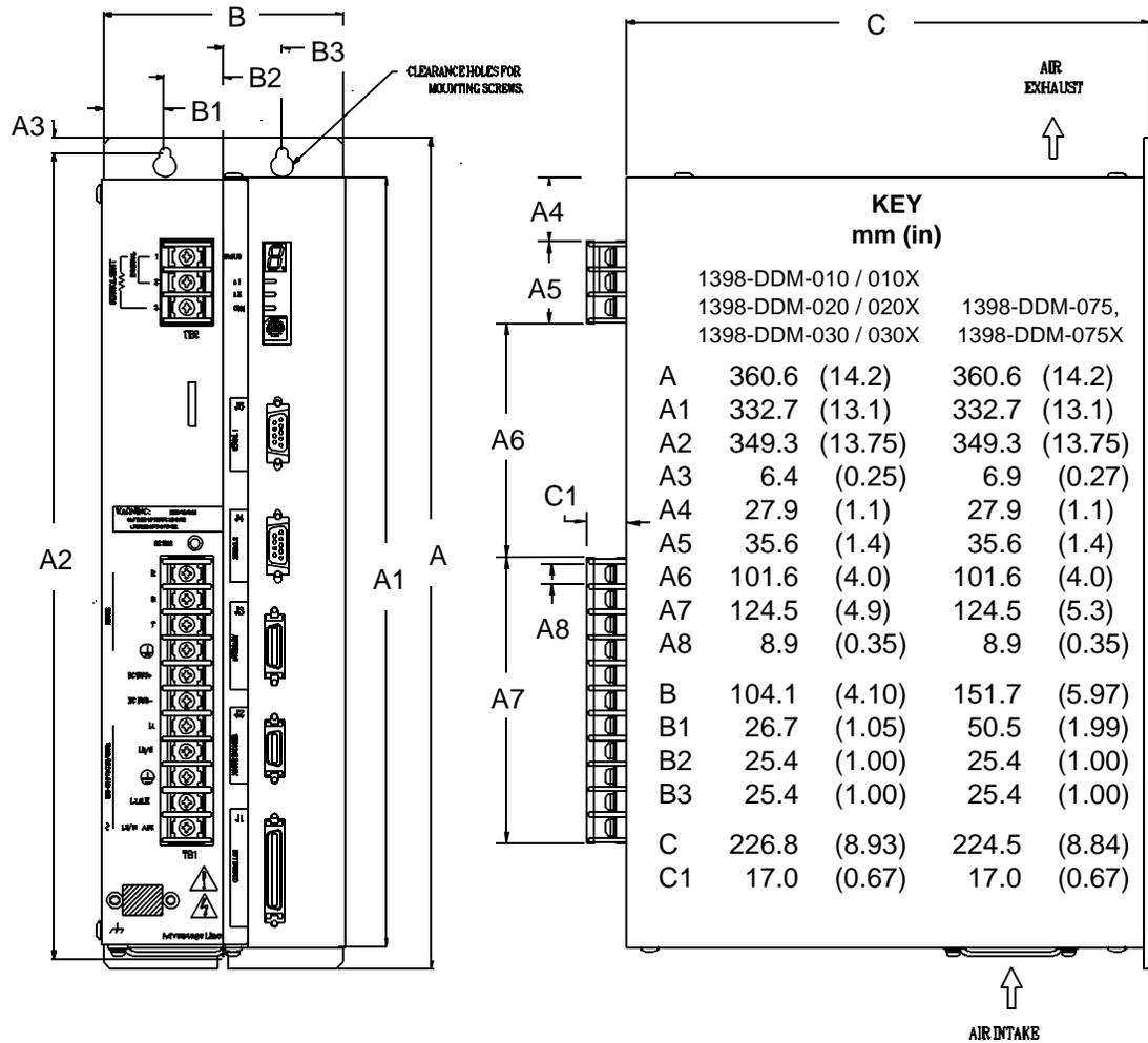
Figure 5.1 1398-DDM Mounting Dimensions (sheet 2 of 2)
