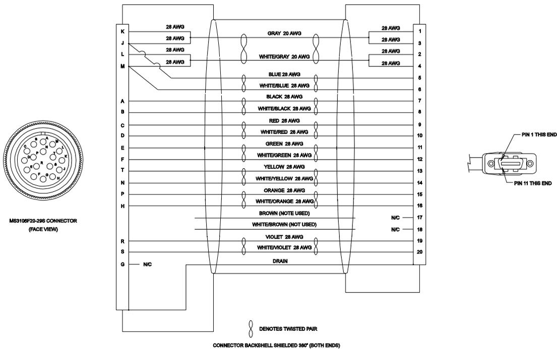
Figure B.14 J2 to Y-Series Encoder Cable (P/N 9101-1375)
