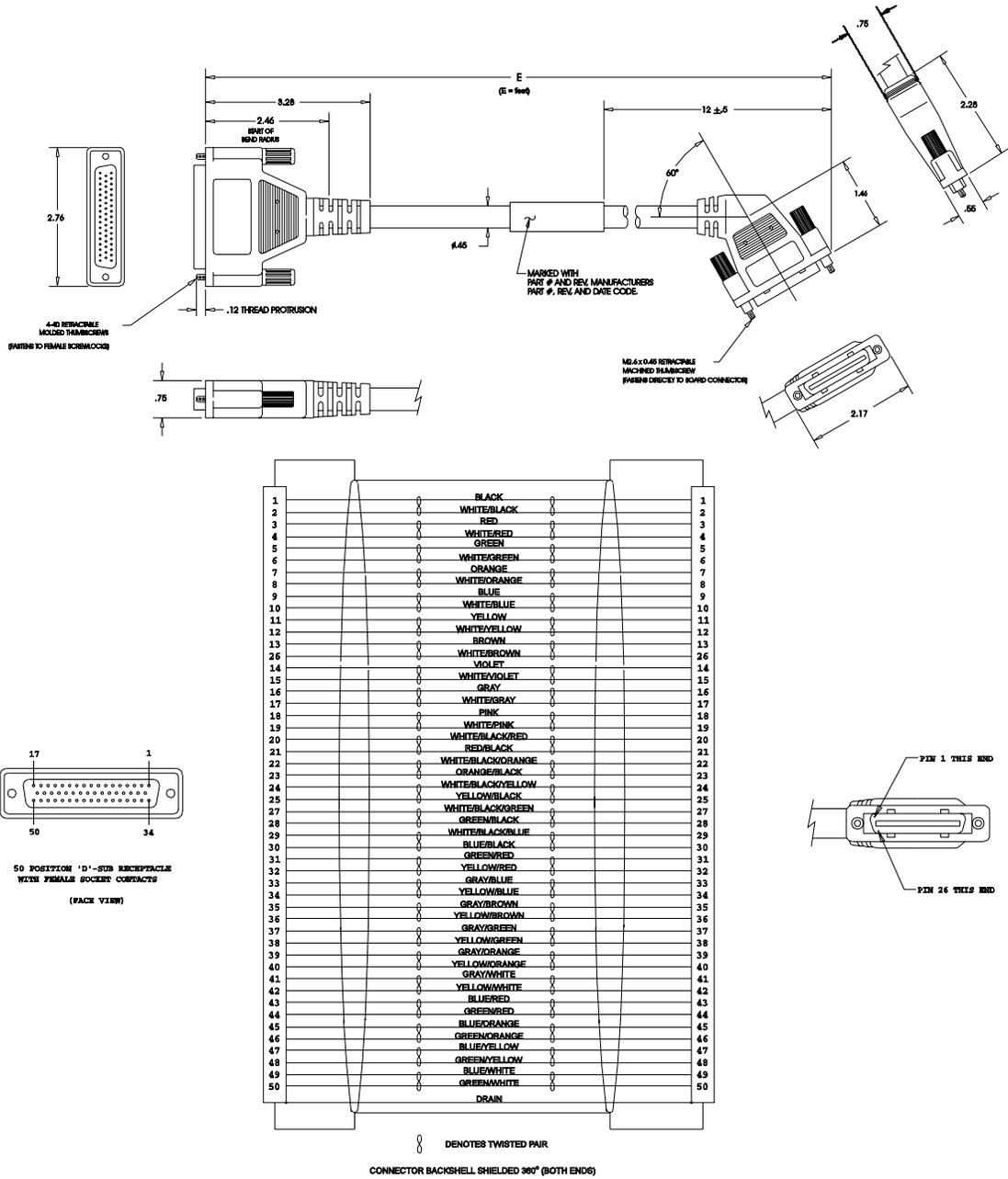
Figure B.7 J2 to 25-pin Terminal Block Kit Diagram (P/N 9101-1392)
