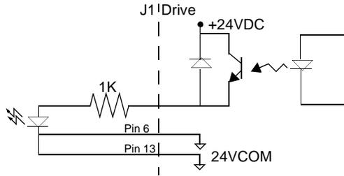
Figure 6.12 Drive Output Connected to a Resistive Load
