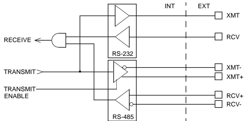
The serial interface of the ULTRA 200 Series uses the standard NRZ asynchronous serial format, and supports both the RS-232 and the four wire RS-485 communications standards.
