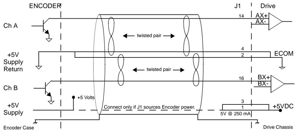
**Figure 6.27 Single-Ended Encoder Interface via Standard TTL Signals (not recommended)**
