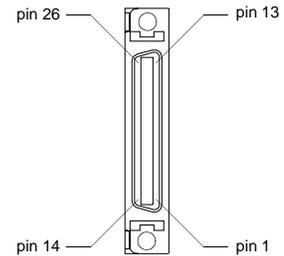
J3 is a 26 pin female mini-D ribbon connector (AMP 2-178238-4). It duplicates the first 26 pins of J1, the Controller connector, which are discussed in detail beginning on page 6-1. Contact between the connector shell and the grounded chassis provides shield termination.
