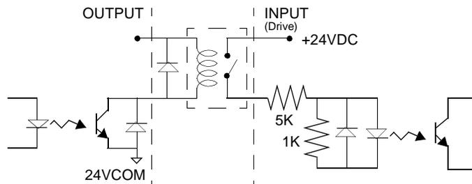
**Figure 6.6 Drive Input Connected to Active Low Output using an Opto-Isolator**
