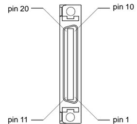
J2 is a 20 pin female mini-D ribbon connector (AMP 2-178238-2). It connects the motor encoder, hall effect switches, and the thermostat to the ULTRA 200 Series drive. Contact between the connector shell and a grounded chassis provides shield termination.
