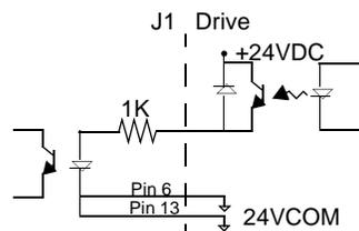
Figure 6.11 Drive Output Connected to an LED Indicator
